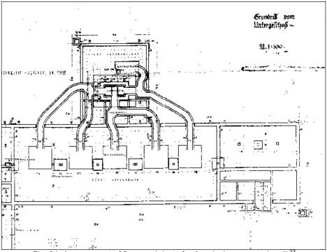
Fig. 34: Arrangement of flues and ducts for Auschwitz crematorium II.<sup>23</sup>
